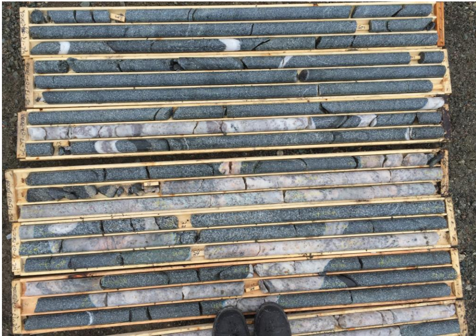
Photo 1 Photo highlighting pegmatite dykes, often spodumene bearing, in hole WL17-07 showing core from 2.6 m to 30.5 m downhole (link to larger version: https://goo.gl/Dv9J5e )
